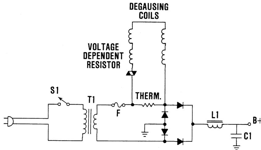
Figure 6.17: AUTOMATIC DEGAUSSING CIRCUIT
