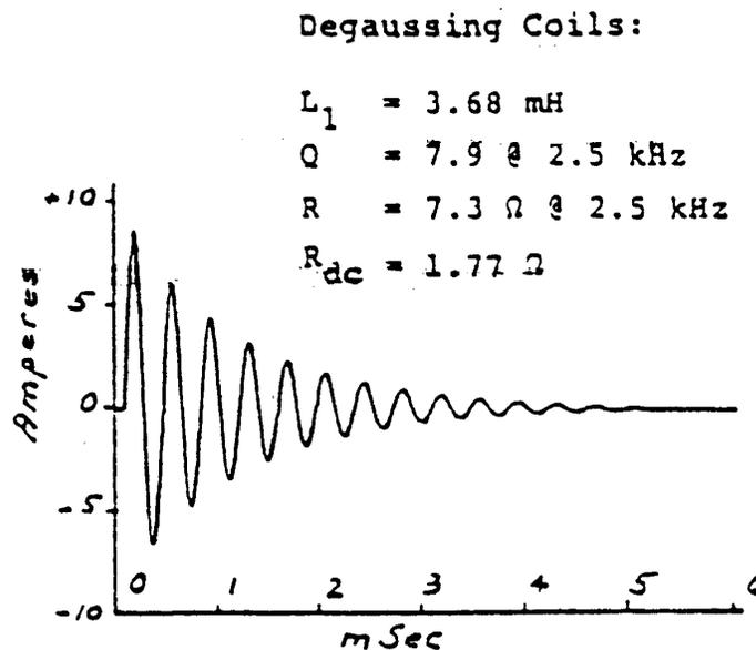
Figure 10: Current in the Degaussing Coils, Side Mounted on a 19V Tube.
