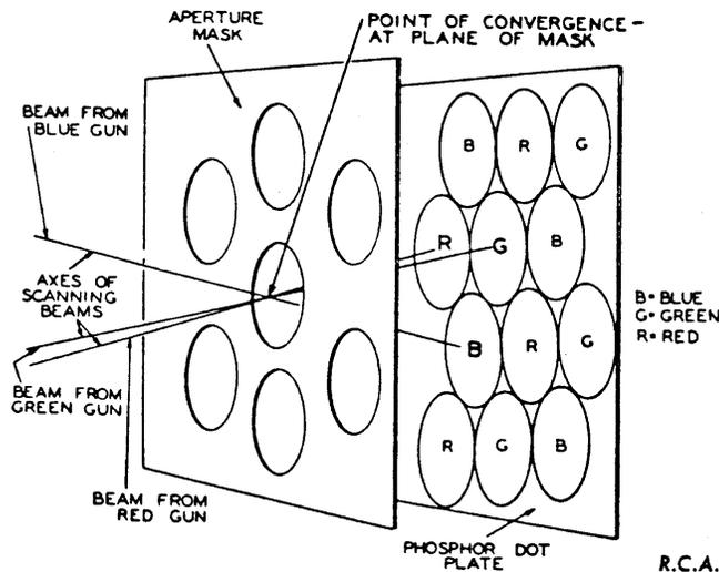
**Figure 6.3:** APERTURE MASK IN DELTA SYSTEM.
